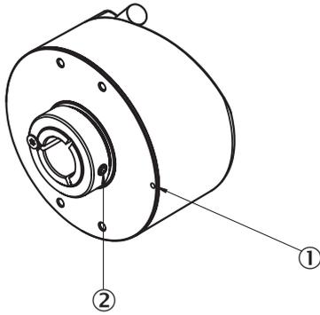
Attention! If stator coupling is mounted, the zero pulse mark can be hidden by the stator coupling
