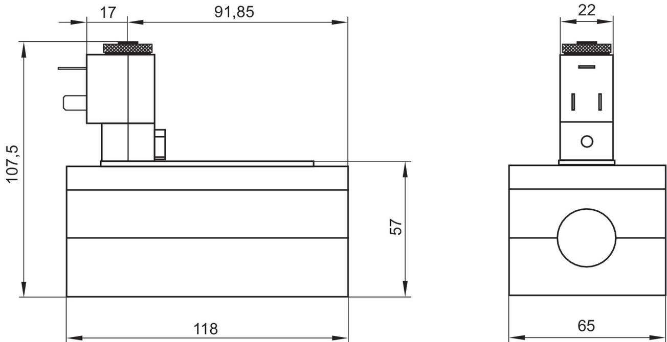
The pilot valves can be loosened and turned through 180°.
