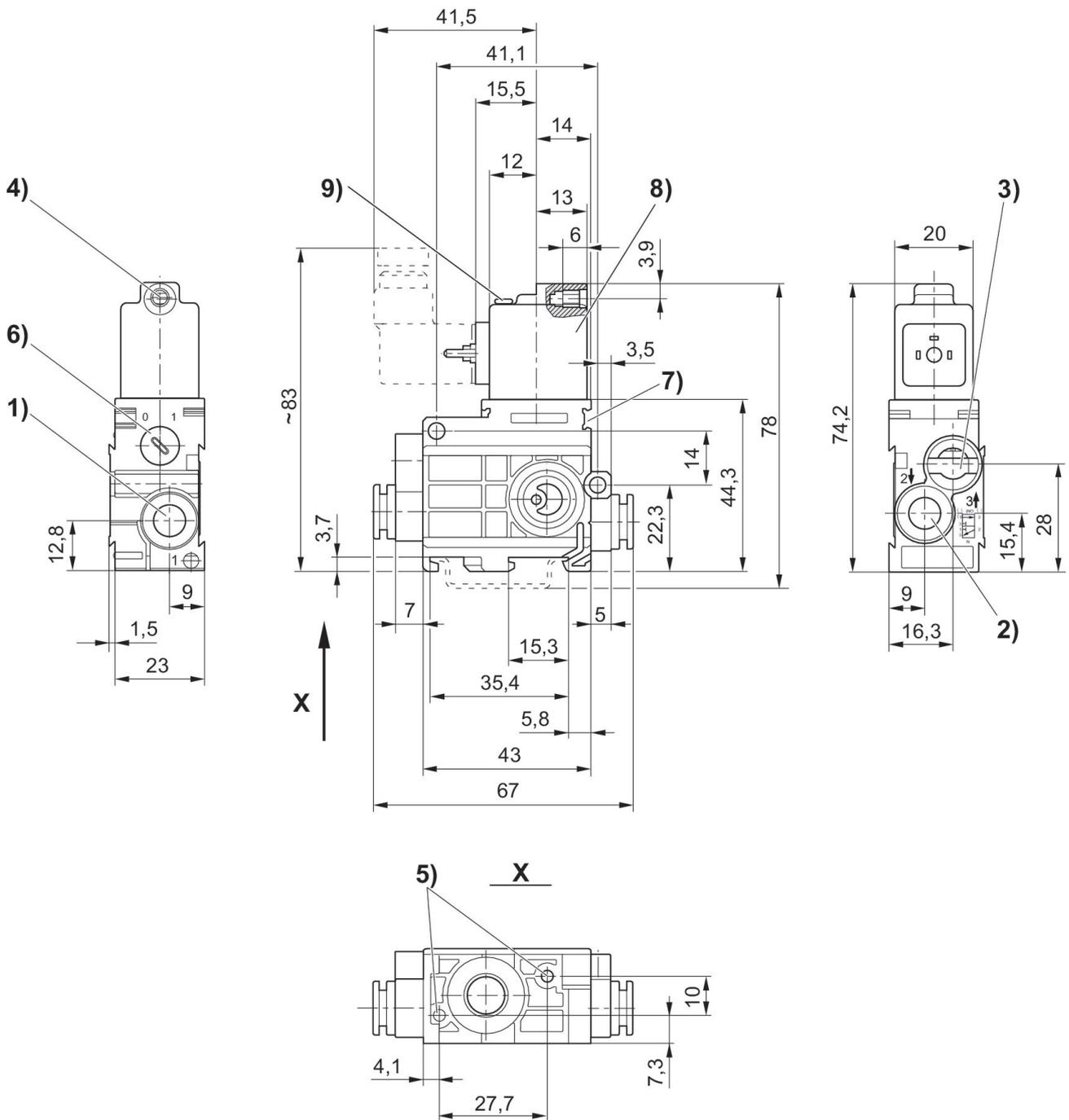
1) Port 1 2) Port 2 3) Port 3, exhaust air must not be throttled 4) Core Ø for M5 5) Pocket hole 6 mm deep for 3.5 self-tapping screw 6) Manual override 7) Mounting space for name plate 8) Coil can be rotated at 180° intervals 9) LED
