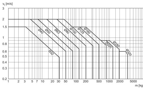
$v_i$  = Piston velocity [m/s]  $m$  = Cushionable mass [kg]
