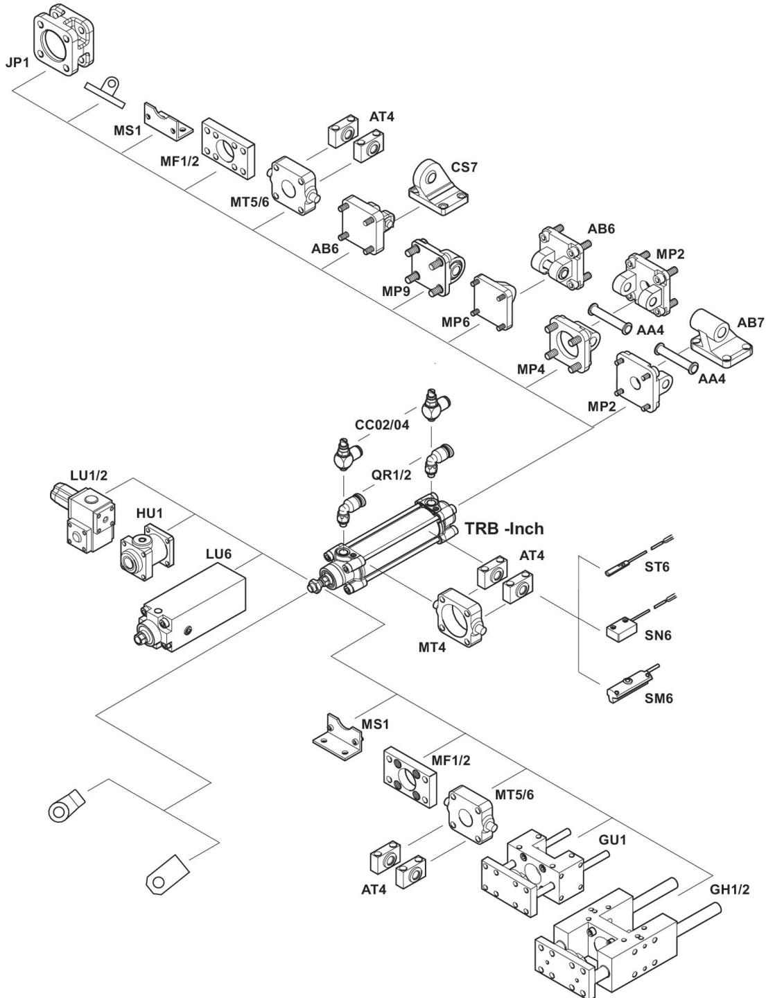
NOTE: This overview drawing is only for orientation to indicate where the various accessory parts can be fastened to the cylinder. The illustration has been simplified for this purpose. It is thus not possible to derive the dimensions from this overview.
