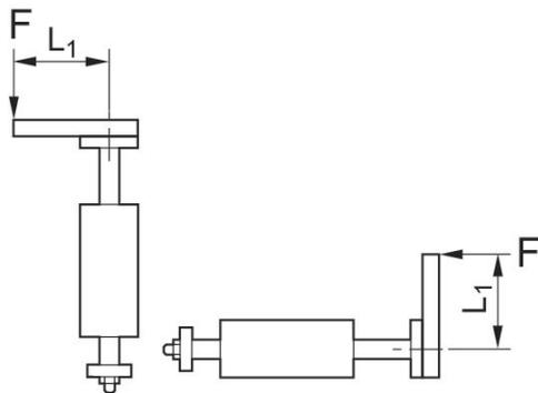
Permissible lever arm length  $L_1$  at 6 bar with static load
