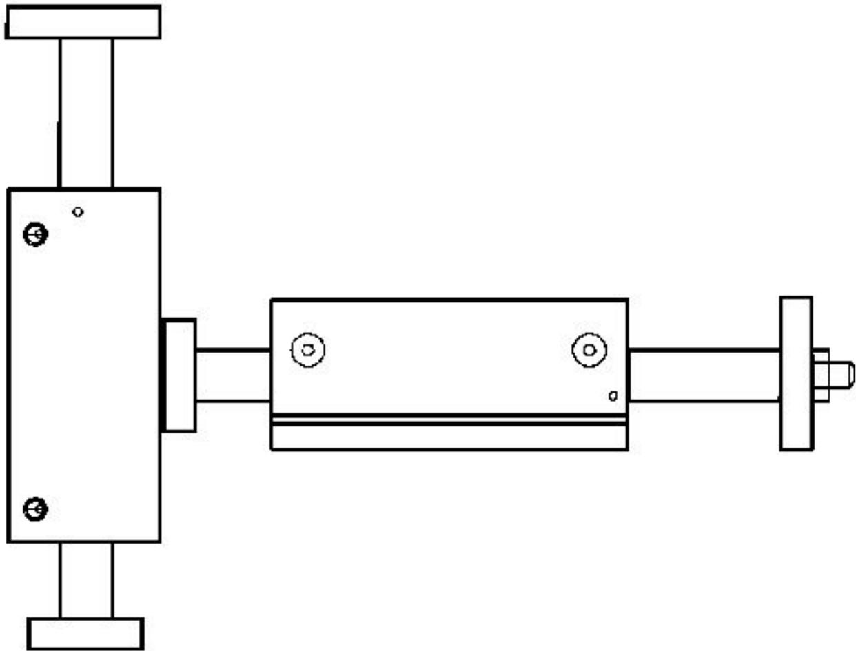
The GPC-E can be directly mounted on the front plate of next bigger standard GPC or GPC-E in radial direction.
