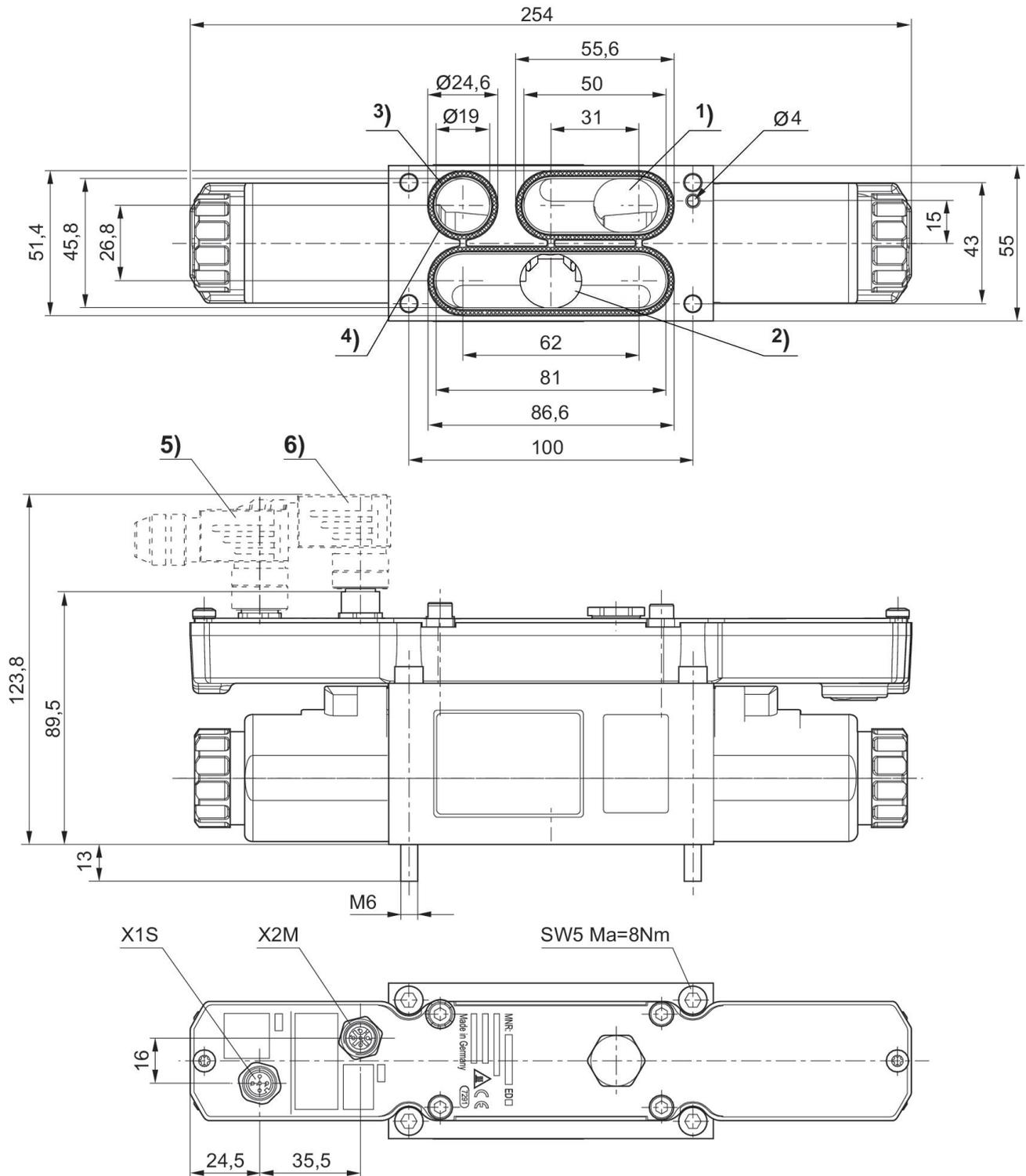
1) Operating pressure 2) Working pressure 3) Exhaust 4) Seal (not assembled) 5) + 6) Accessories not supplied
