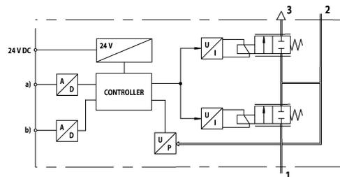
a) Nominal input value b) Actual output value The E/P pressure control valve modulates the pressure corresponding to an analog electrical nominal input value.
