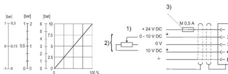
1) Supply voltage 2) Potentiometer supply (pin 4) and nominal value (pin 2) are related to 0 V. Potentiometer resistance min. 0-2 kΩ, max. 0-10 kΩ. 3) The operating voltage must be protected by an external M 0.5 A fuse. Connect the plug via a shielded cable to ensure EMC.
