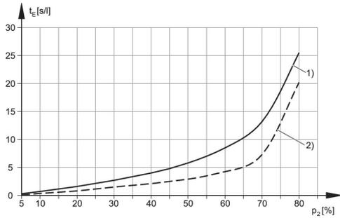
1) =  $\varnothing$  nozzle 0.5 mm 2) =  $\varnothing$  nozzle 0.7 mm
