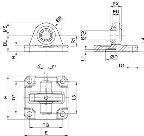
Scope of delivery: clevis incl. mounting screws
