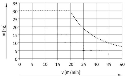
Max. permissible radial bearing load F
