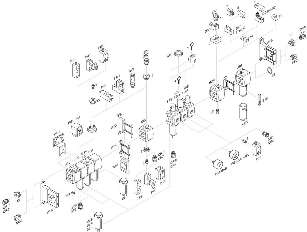
1 = contamination display 3 = Double nipple 4 = Key for E11 locking 5 = mortise lock 6 = Transition plate DO30 7 = Adapter, Series CON-VP 8 = Mounting aid DO16, form C 9 = Mounting aid DO16, M12 10 = Adapter for external pilot air 11 = Adapter pneumatic operation 12 = Sealing ring 13 = Reducing nipple
