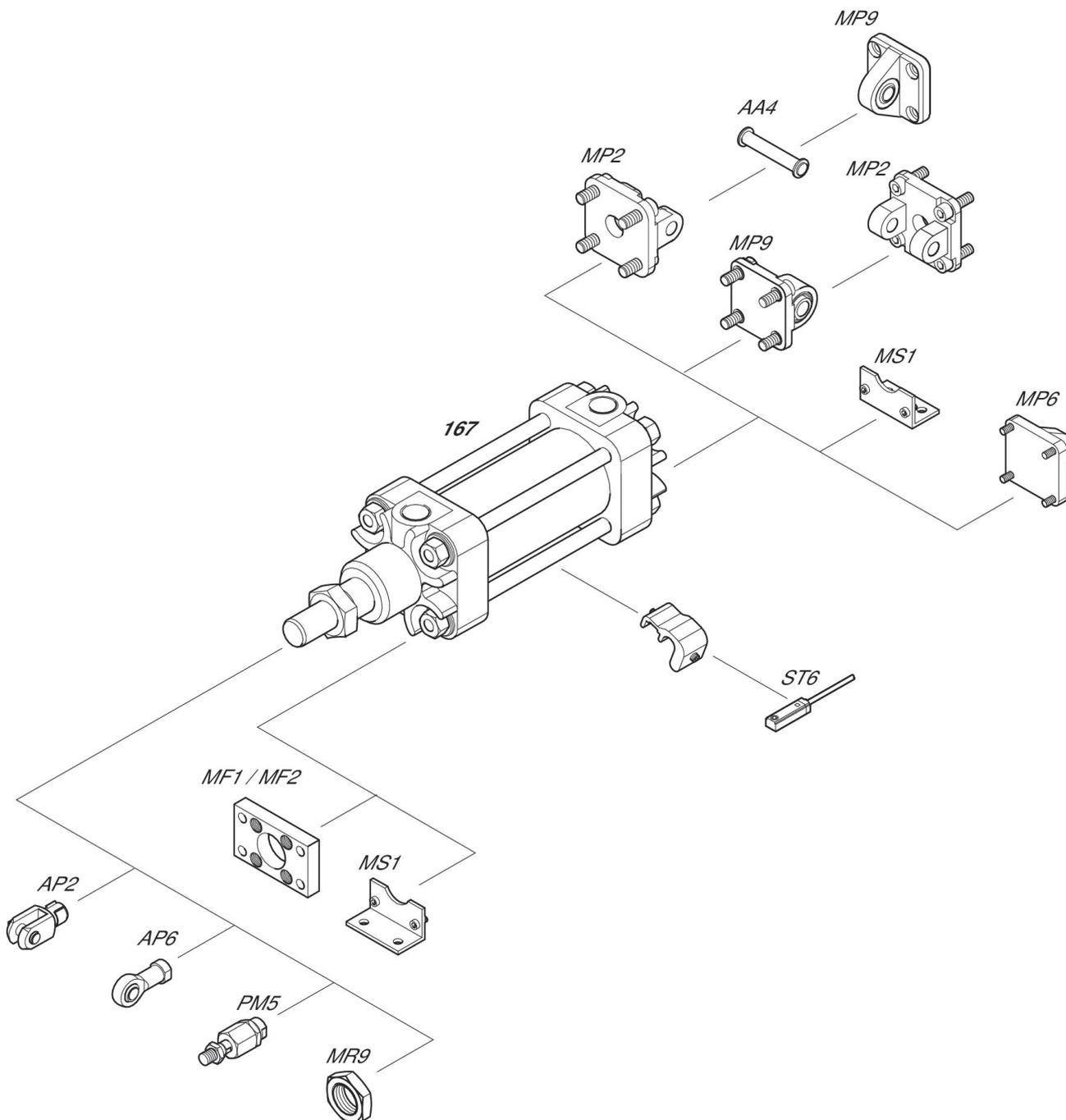
NOTE: This overview drawing is only for orientation to indicate where the various accessory parts can be fastened to the cylinder. The illustration has been simplified for this purpose. It is thus not possible to derive the dimensions from this overview.
